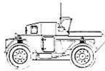
MV/2 DAIMLER 'DINGO' SCOUT CAR (WORLD WAR II) This Daimler scout car, popularly known as the 'Dingo', saw service in many theatres of war with British and Commonwealth forces during and after the Second World War, as a command, reconnaissance or communications vehicle. Armament was normally provided by a .303 Bren L.M.G. which was fixed to fire through a vertical slot in the turret front plate.
